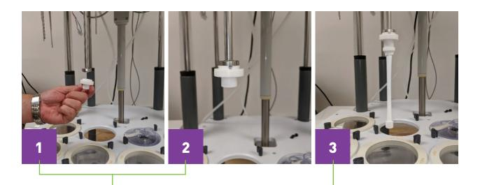
First install the Float-A-Lyzer® Holder onto a basket shaft. Attach the desired Float-A-Lyzer® into the holder. Then in a dry vessel, align the Float-A-Lyzer® Holder to the correct height by adjusting the basket shaft position for any of the FLTHLD-BSKxx adapters.
