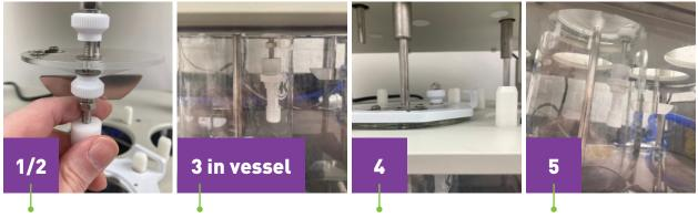
Set the paddle height for the dissolution tester and lower the drive head into the testing position.
